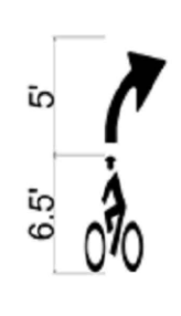
PAVEMENT MARKING EPOXY, SPECIAL BIKE SYMBOL WITH RIGHT ARROW SEE SHEET M-7 AND SPECS
